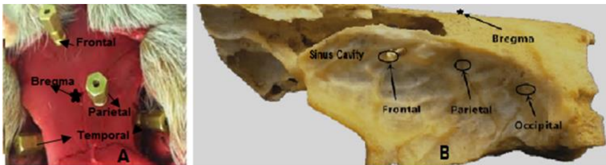
Figure 3-18: (A) A snapshot showing the locations of installed mounts for pressure transducer installation and (B) A sectional view of a skull which shows the frontal sinus cavity along with corresponding frontal sensor location.
